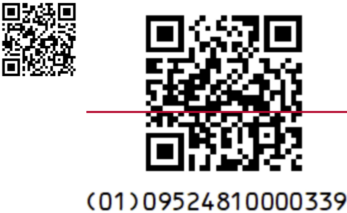
Figure C.1 — Example of QR code encoding a GS1 identifier in an ISO/IEC 18975 compliant: GS1 Digital Link URI Example of a structured path URI that uses GS1 Application Identifiers
