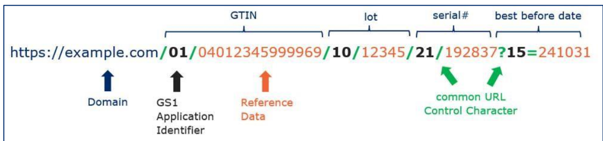
Figure 2.2-1: Method 1: Web-enabled, structured path, GS1 identifiers
