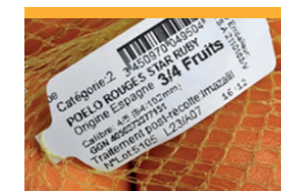
Figure 3-13. Example Scanning issue due to lack of height
